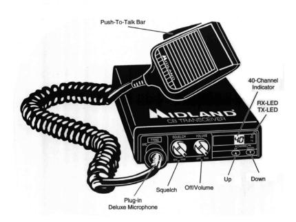
**ON/OFF VOLUME:** In the off position your transceiver power is off. Turn this control clockwise to switch on the unit and adjust the volume.
